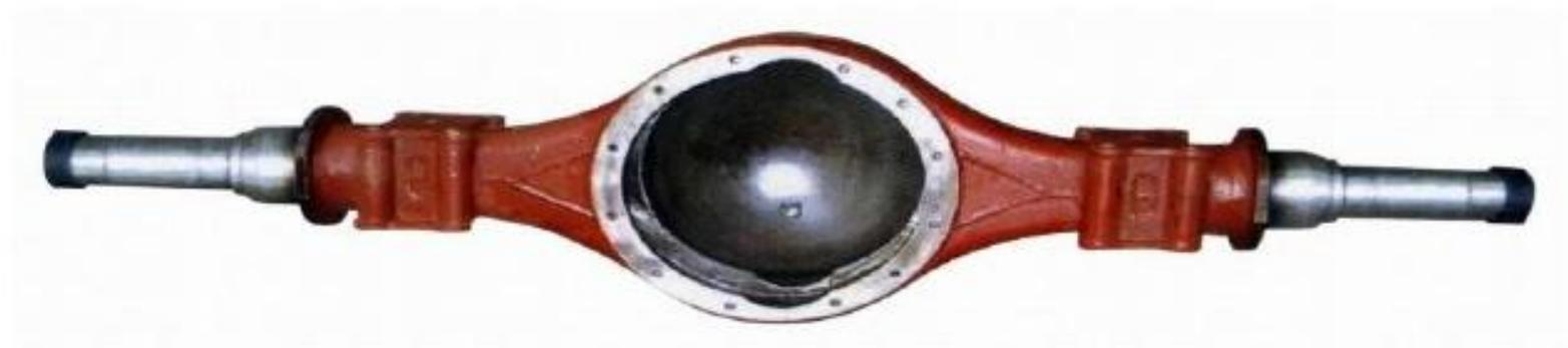
Fig: Mercedes Benz Rear Axle Housing (Banjo Type)
